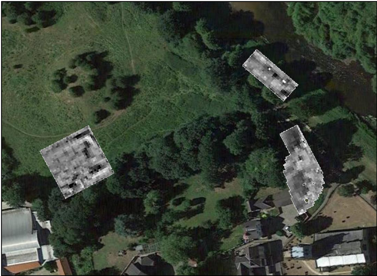
Figure 6. Results of resistivity surveys at the three locations. (Map data © Google, 2018).
